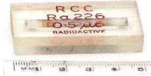
Clear block with metal strip (Ra226)
