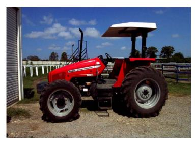
Queensland legislation requires tractors at workplaces (including schools) manufactured after 1 January 1981 to be fitted with a Rollover Protective Structure (ROPS).
