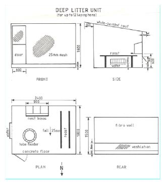
Figure 1: A shed for up to 12 laying hens. A similar shed without the nest boxes and roost would suit meat chickens. (All measurements are in mm.)
