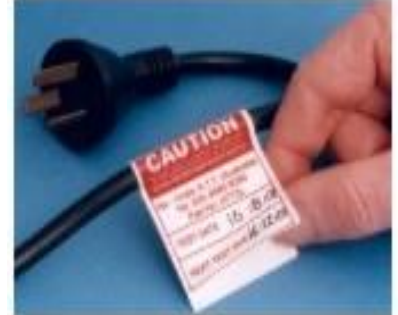
The label (tag) attached to the item specifies the next test date.
