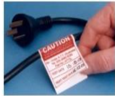
The label (tag) attached to the item specifies the next test date.
