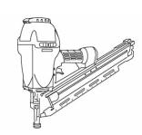
Nailing gun Average noise level 95dB Possible hearing damage after 45 sec
